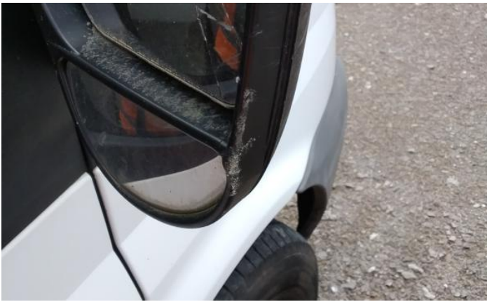
27: Door osf Scratched Over 25mm Thru Paint
