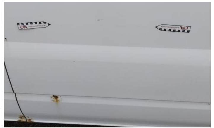
22: Qtr Panel osr Scratched Over 25mm Not Thru Paint
