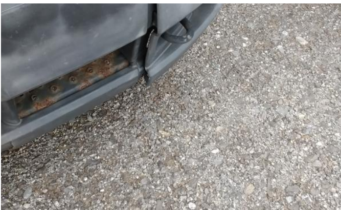
5: Screen Front Chipped Over 10mm
