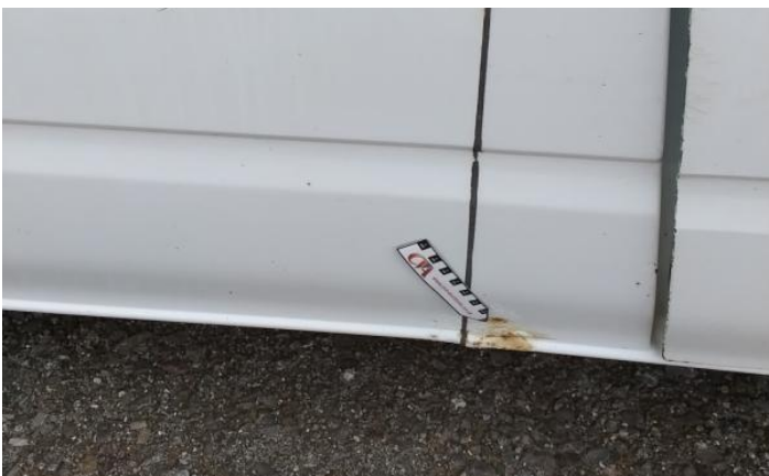
23: Qtr Panel osr Rusted Over 5mm
