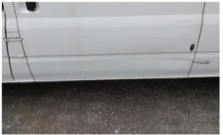
10: Door nsf Dented 2 Or Less Up To 10mm
