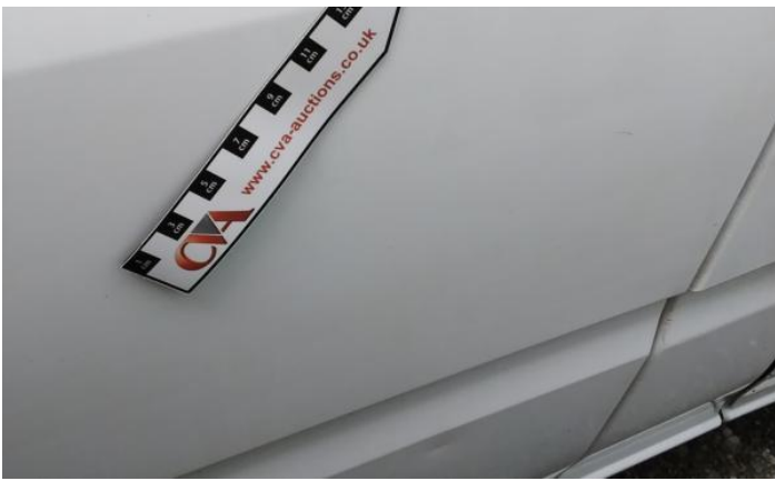
9: Wing nsf Scratched Over 25mm Thru Paint
