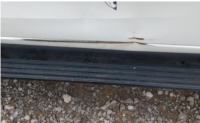
11: Panel Rear Cracked Replace
