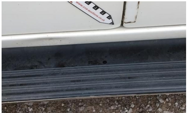
6: Sill ns Dented With Paint Damage
