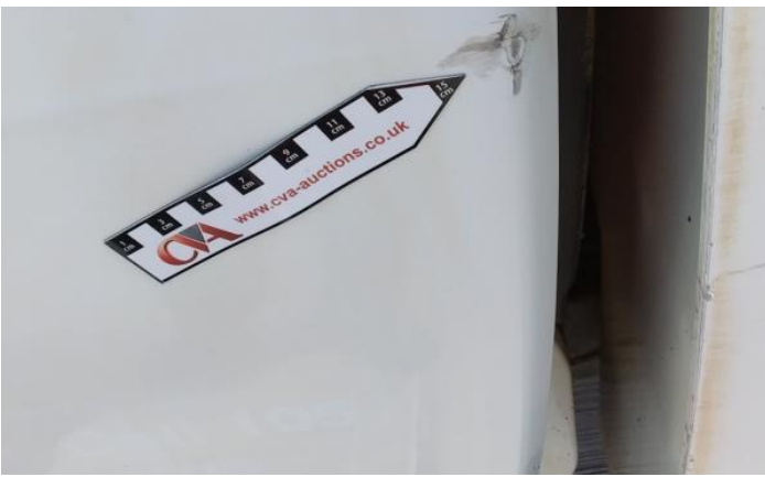
9: Sill ns Scratched Over 25mm Thru Paint
