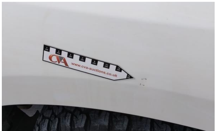
16: Door osf Dented With Paint Damage
