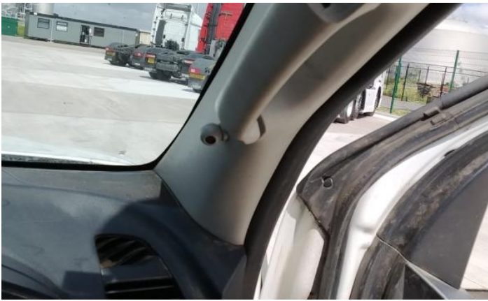
21: Centre Console Front Holed Over 3mm
