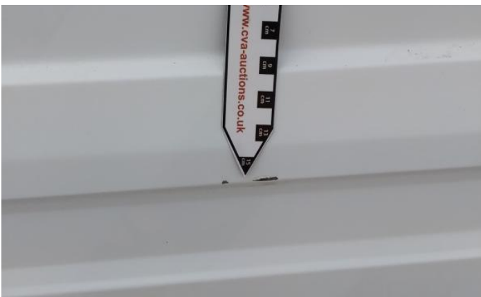
23: Bumper Rear Scratched 25 to 100mm Thru Paint
