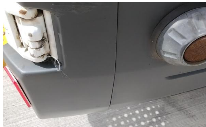
21: Door osr Dented Between 10mm + 30mm
