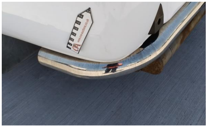
10: Qtr Panel nsr Chipped Over 5mm
