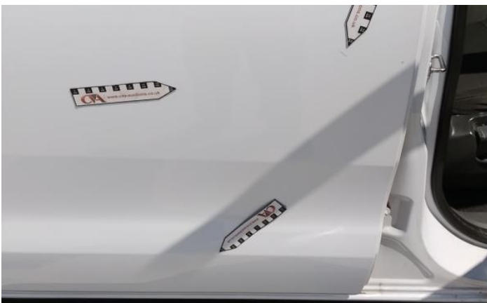
17: Qtr Panel osr Poor Previous Repair Paint Flake
