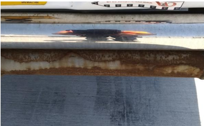
11: Qtr Panel nsr Dented With Paint Damage
