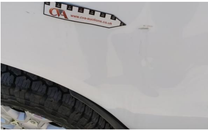
9: Qtr Panel nsr Scratched Over 25mm Thru Paint
