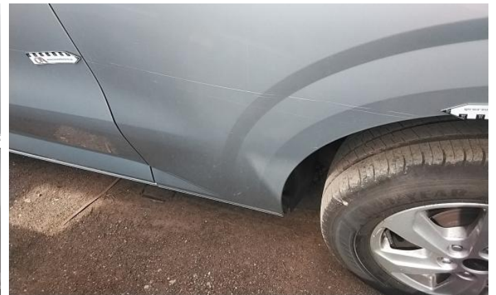
6: Fuel Flap Scratched Over 25mm Thru Paint
