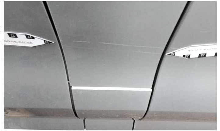
4: Door nsf Scratched Over 25mm Thru Paint
