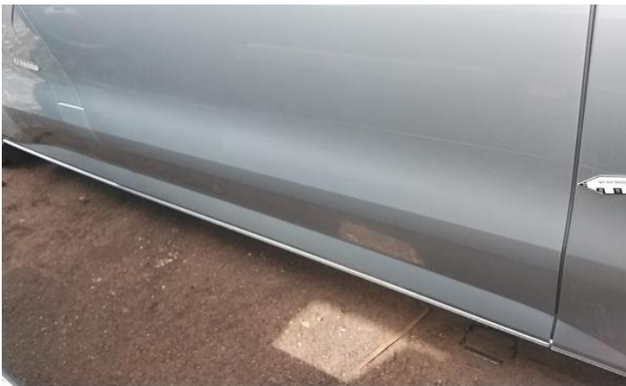
5: Door nsf Scratched Over 25mm Thru Paint
