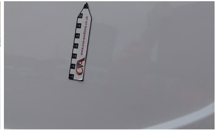
16: Qtr Panel osr Dented Between 10mm + 30mm
