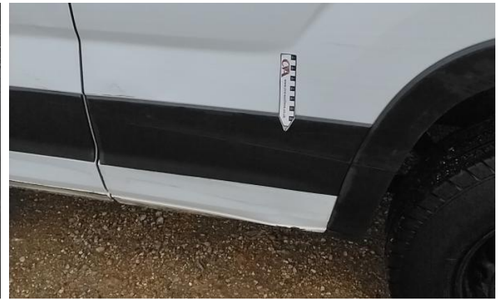
16: Sill ns Dented With Paint Damage
