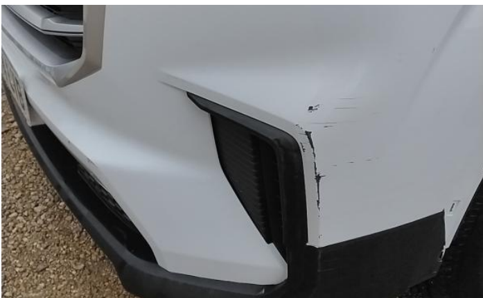
5: Bumper Front Scratched 25 to 100mm Thru Paint
