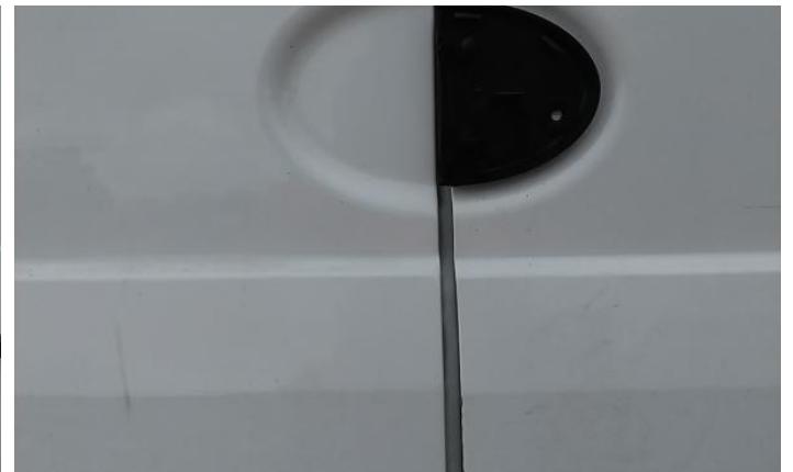
18: Qtr Panel Moulding ns Scuffed (Unpainted) Up To 100mm
