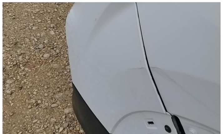
6: Bumper Front Scratched 25 to 100mm Thru Paint
