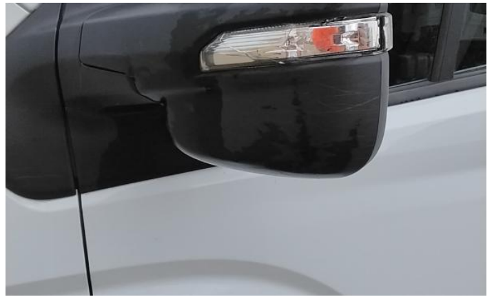
10: Wing nsf Scratched Over 25mm Not Thru Paint
