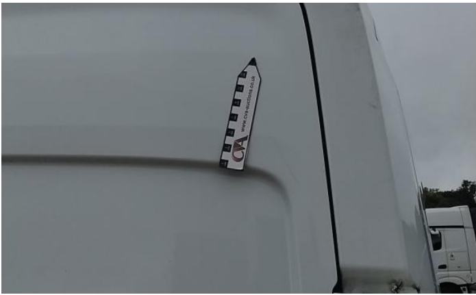
21: Door osr Dented With Paint Damage
