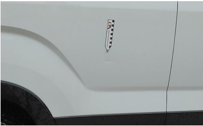
9: Door nsr Dented With Paint Damage
