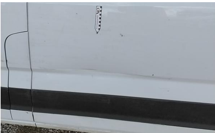
5: Door Moulding nsf Scuffed (Unpainted) Over 100mm
