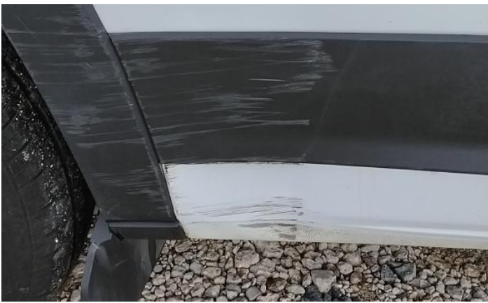
3: Wing Front Arch Extension ns Scuffed (Unpainted) Over 100mm
