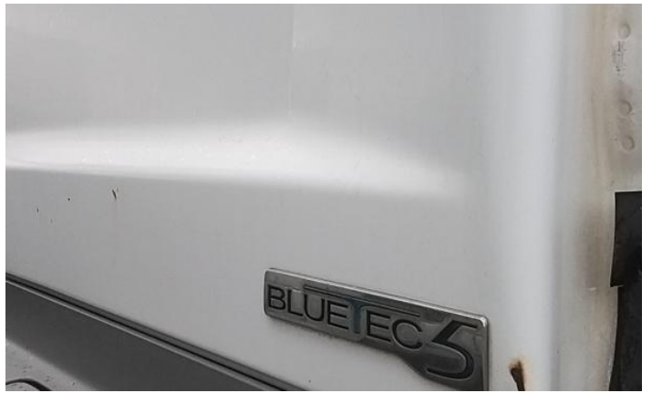
4: Panel Rear Rusted Over 5mm
