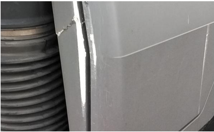
3: Door osf Scratched Over 25mm Thru Paint
