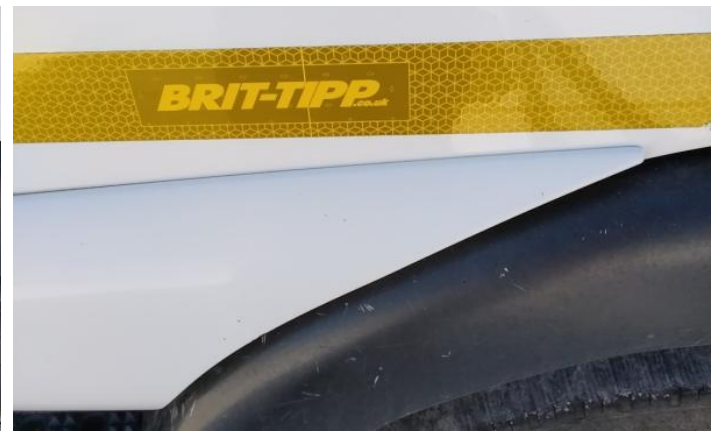
4: Door nsf Scratched Over 25mm Thru Paint
