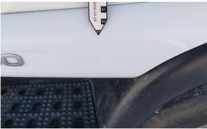
3: Moulding nsf Wing Scratched (Painted) Over 25mm Thru Paint
