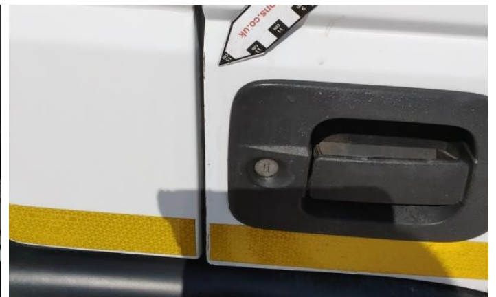
6: Door nsf Scratched Over 25mm Thru Paint
