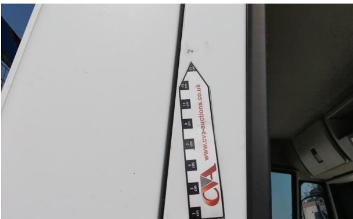
5: Door nsf Scratched Over 25mm Thru Paint
