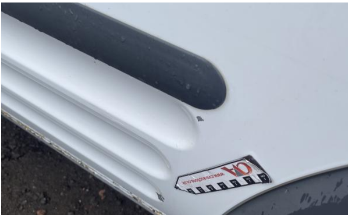
5: Qtr Panel osr Dented With Paint Damage
