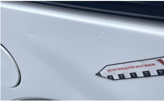
3: Door osf Dented With Paint Damage
