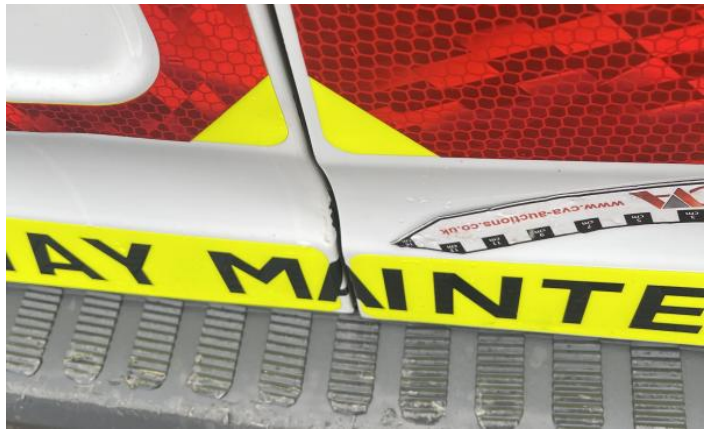
4: Door osr Rusted Over 5mm
