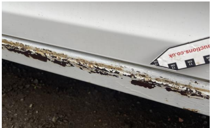
6: Tailgate Rusted Over 5mm
