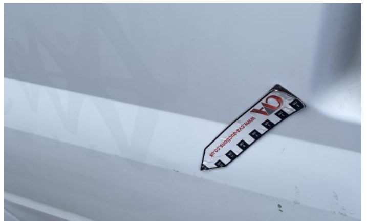
10: Door nsr Dented With Paint Damage
