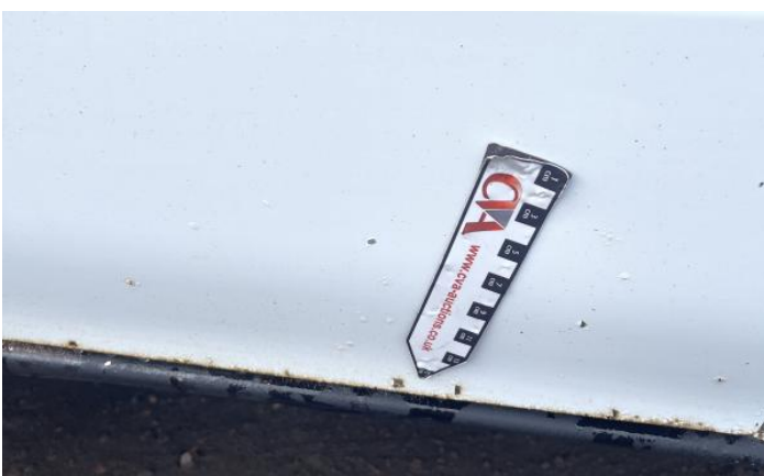
11: B Post ns Rusted Over 5mm
