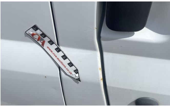
3: Wing osf Dented With Paint Damage
