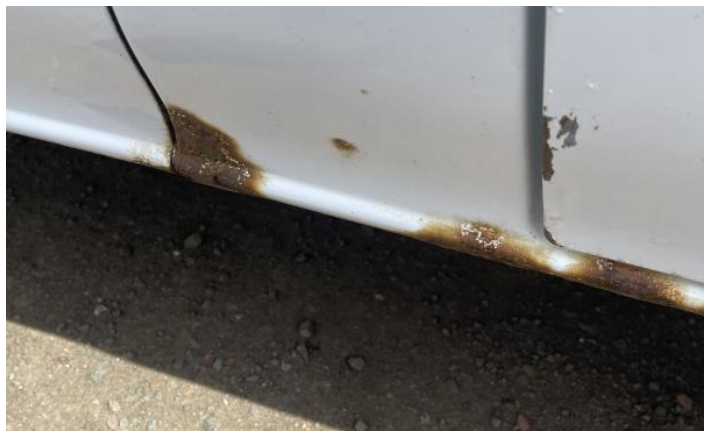
4: Door osf Rusted Over 5mm
