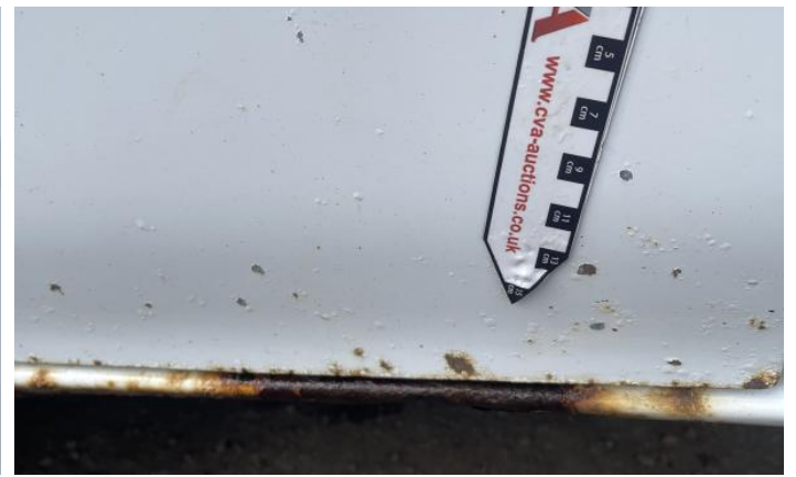
10: B Post ns Rusted Over 5mm
