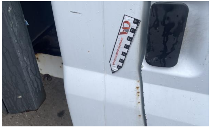
4: Wing osf Rusted Over 5mm
