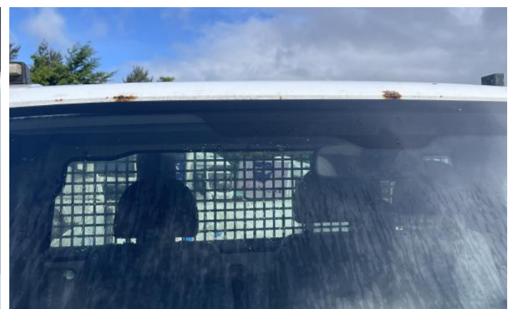
12: Sill ns Rusted Over 5mm
