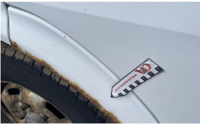
9: Qtr Panel nsr Dented With Paint Damage
