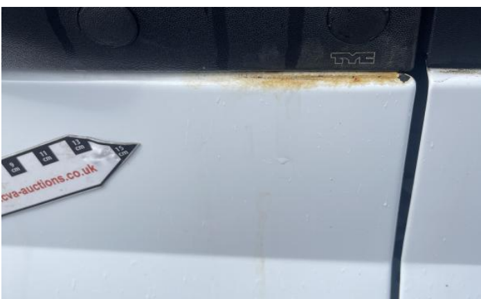
11: Door nsf Rusted Over 5mm
