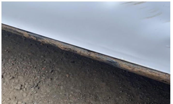
10: Qtr Panel nsr Rusted Over 5mm
