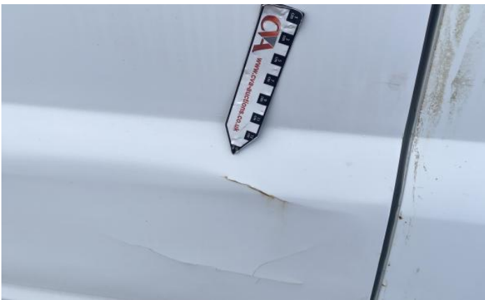
9: Tailgate Dented With Paint Damage
