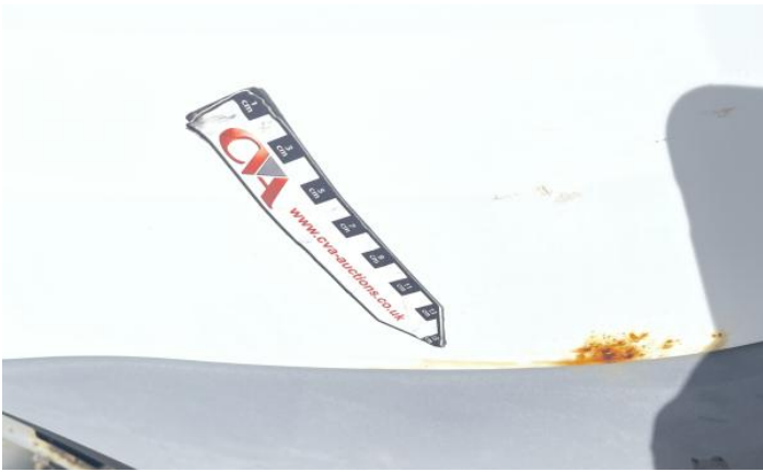
3: Roof Rusted Over 5mm
