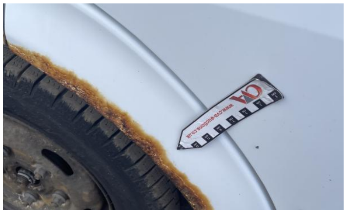
12: Sill ns Rusted Over 5mm
