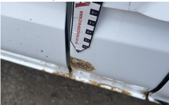
11: Door nsr Dented With Paint Damage
