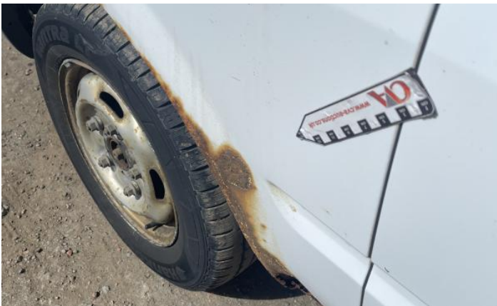
5: Wing of Rusted Over 5mm
