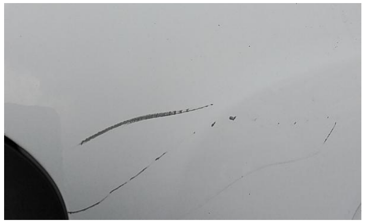
4: Qtr Panel osr Scratched Over 25mm Thru Paint
