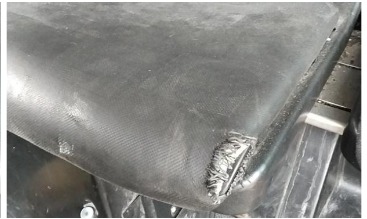
10: Seat Base Cover osf Torn Over 3mm
