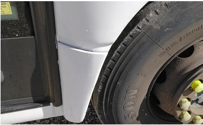
3: Bumper Front Scratched 25 to 100mm Thru Paint
