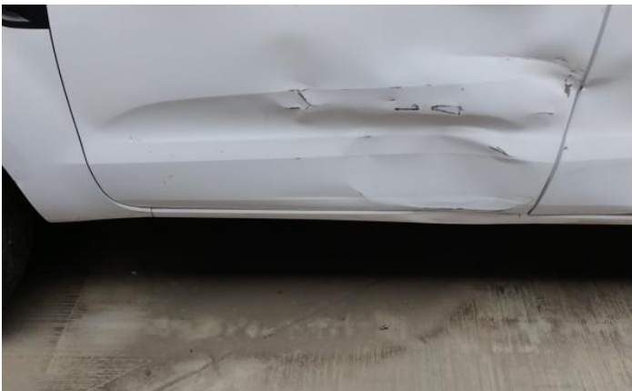
5: Wing nsf Dented Hail - Severe
