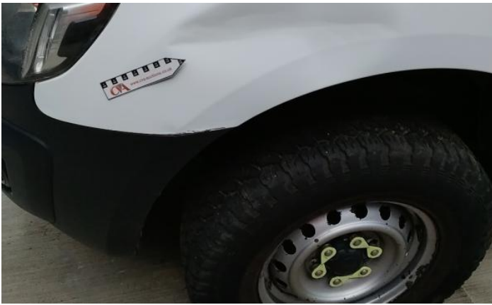
3: Bonnet Dented Over 30mm
