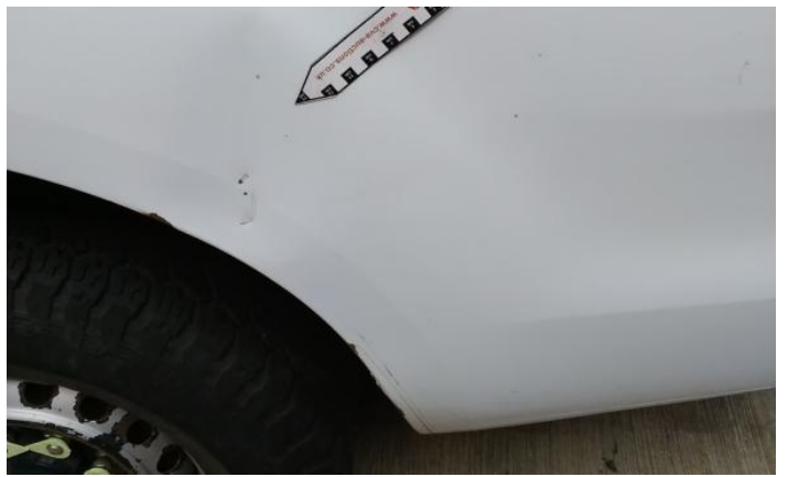
10: Sill ns Dented Over 30mm
