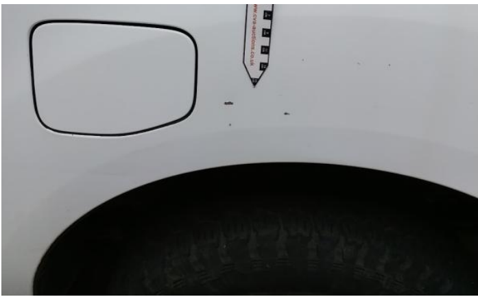
9: Qtr Panel nsr Dented Over 30% Of Panel
