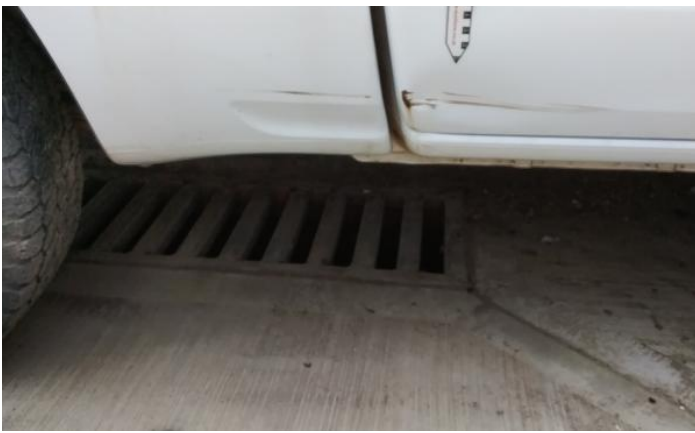
15: Qtr Panel osr Dented With Paint Damage
