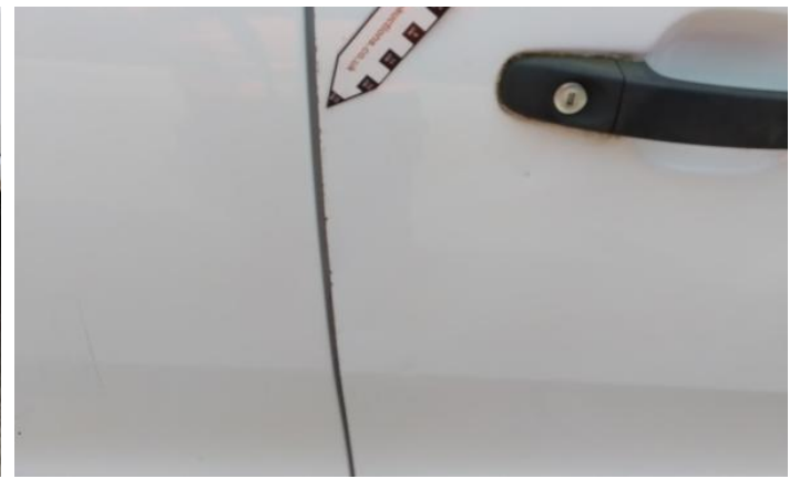
16: Qtr Panel osr Scratched Over 25mm Thru Paint
