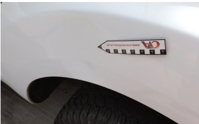
17: Qtr Panel osr Scratched Over 25mm Thru Paint
