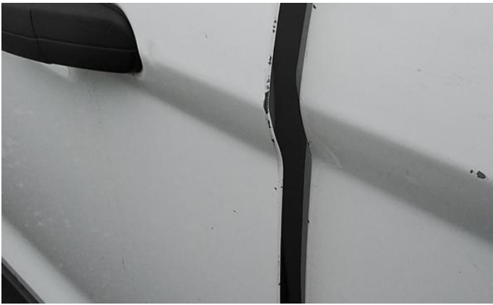
9: Panel Rear Dented With Paint Damage
