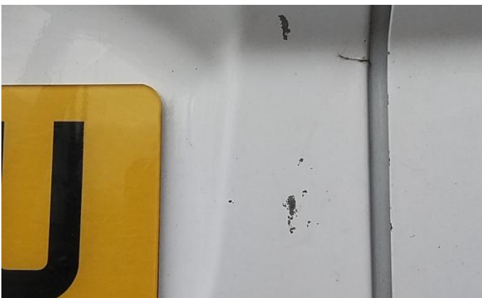
5: Panel Rear Scratched Over 25mm Thru Paint
