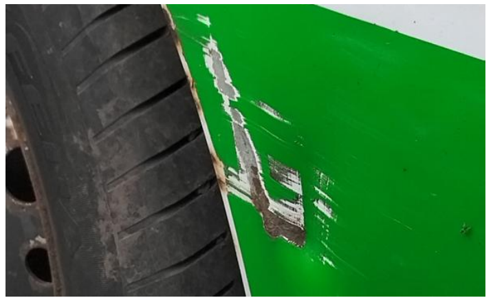
4: Panel Rear Scratched Rusted
