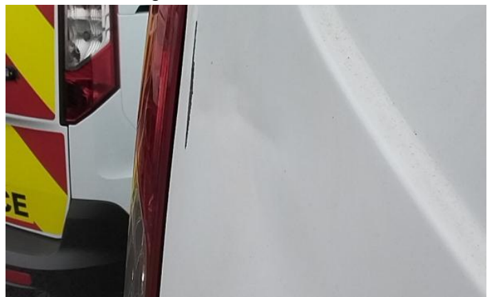
6: Panel Rear Dented With Paint Damage
