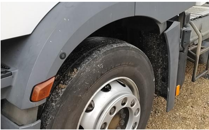
3: Bumper Front Moulding Scuffed (Unpainted) Over 100mm
