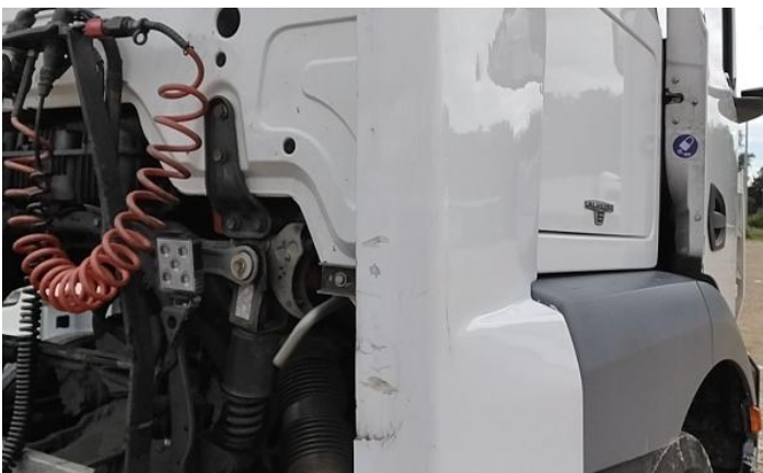
5: Wing Front Arch Extension ns Scratched (Painted) Over 25mm Thru Paint
