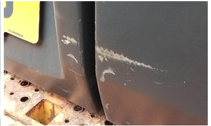
4: Panel Rear Scratched Over 25mm Not Thru Paint
