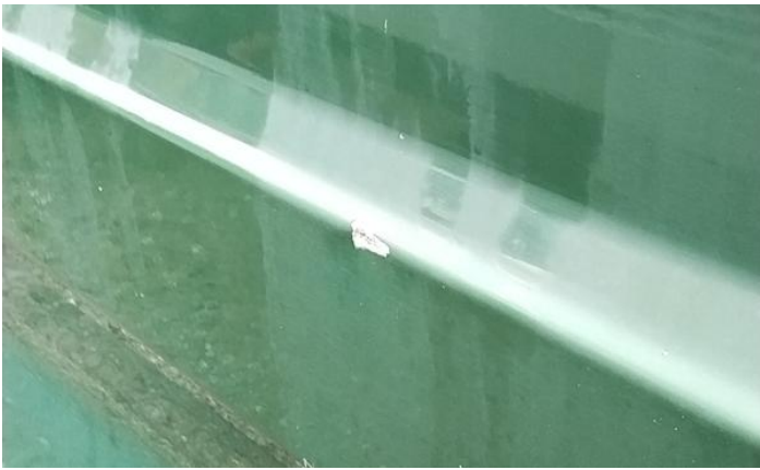
3: Sill os Scratched UpTo 25mm Not Thru Paint
