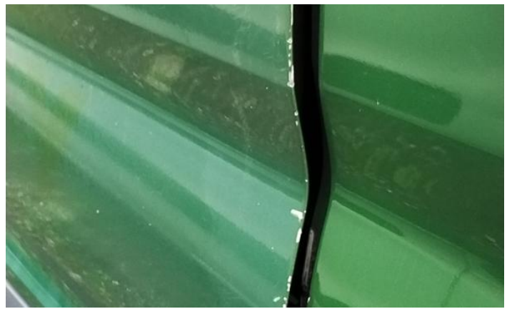
10: Door nsr Scratched Over 25mm Not Thru Paint
