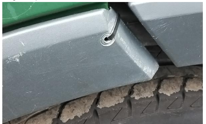
12: Door nsf Chipped Edge Chip
