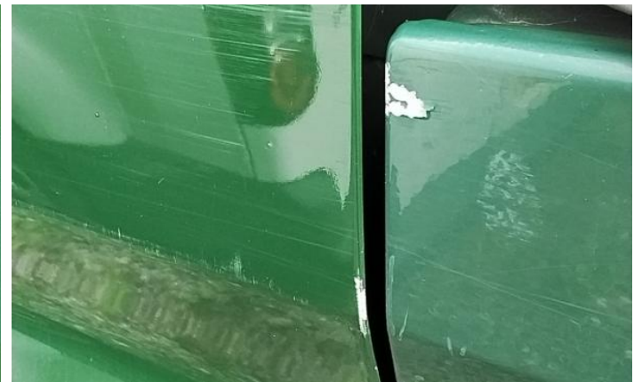
6: Tailgate Trim Panel Scuffed (Unpainted) Over 100mm
