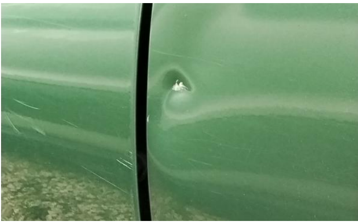
3: Bumper Rear Moulding Scuffed (Unpainted) Up To 100mm
