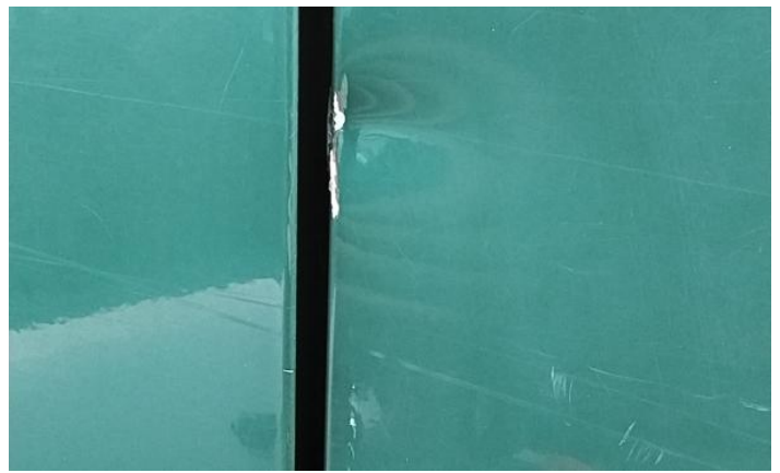
4: Panel Rear Scratched Over 25mm Thru Paint
