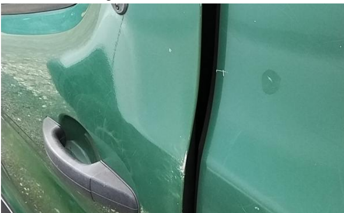
5: Panel Rear Dented With Paint Damage
