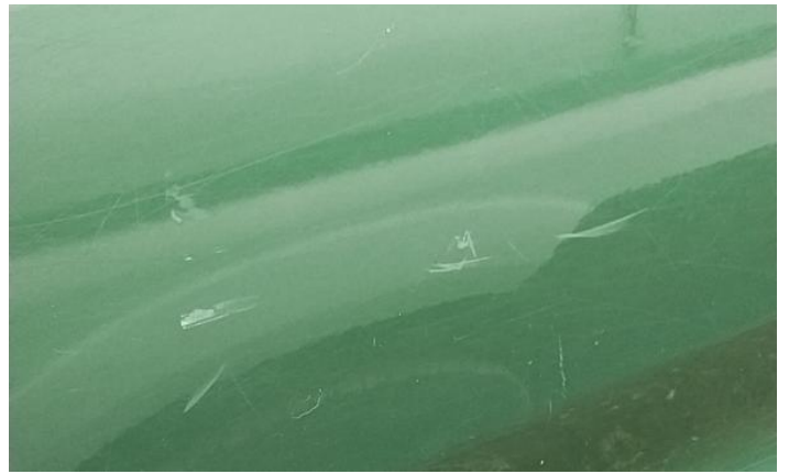
10: Door nsf Chipped Multiple Chips
