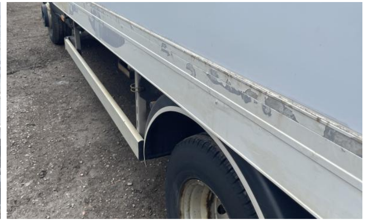
4: Qtr Panel osr Rusted Over 5mm
