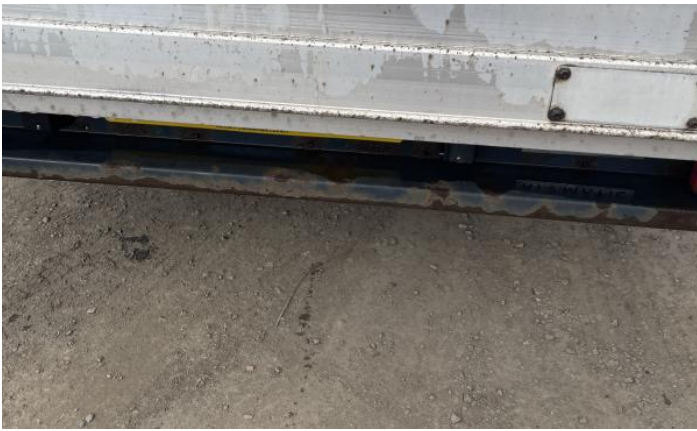
3: Wing osf Dented With Paint Damage
