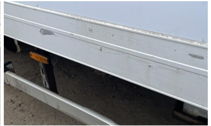
4: Qtr Panel osr Rusted Over 5mm
