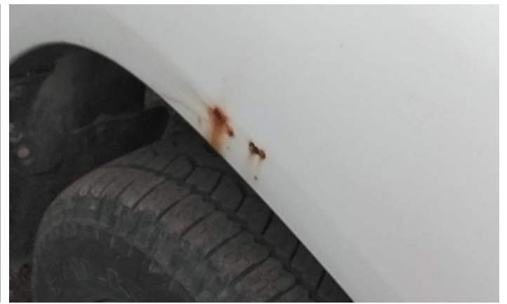
4: Sill os Scratched Over 25mm Thru Paint
