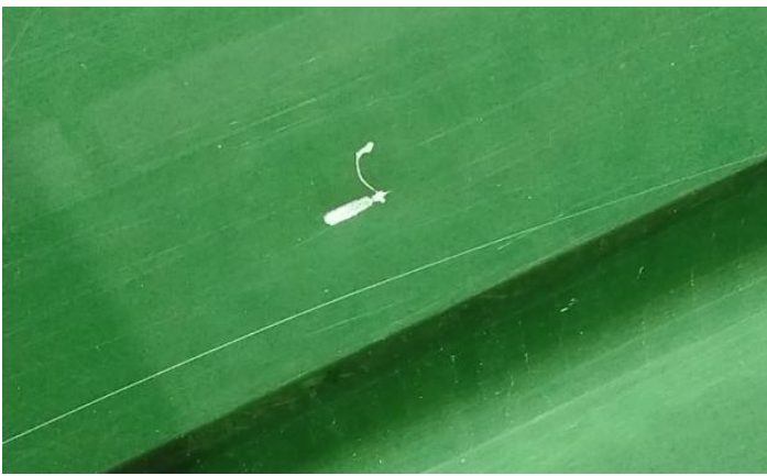
9: Panel Rear Scratched Over 25mm Not Thru Paint
