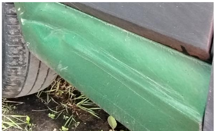
6: Door nsr Scratched Over 25mm Not Thru Paint
