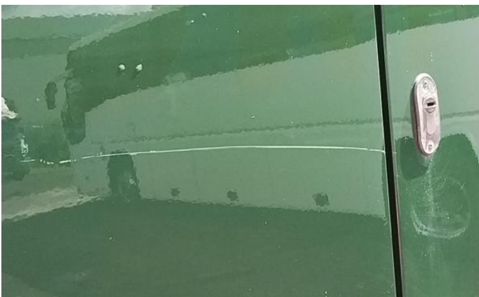
5: Panel Rear Scratched Over 25mm Thru Paint
