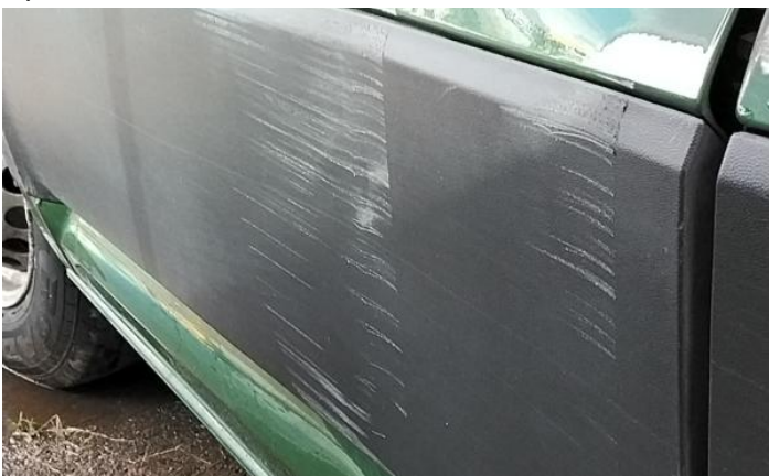
11: Panel Rear Scratched Up To 25mm Thru Paint
