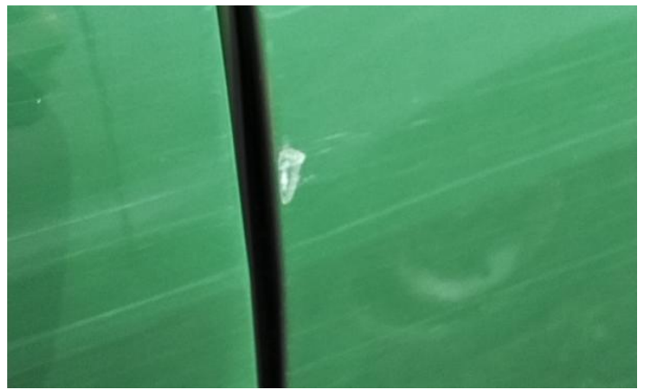
10: Panel Rear Scratched Over 25mm Not Thru Paint
