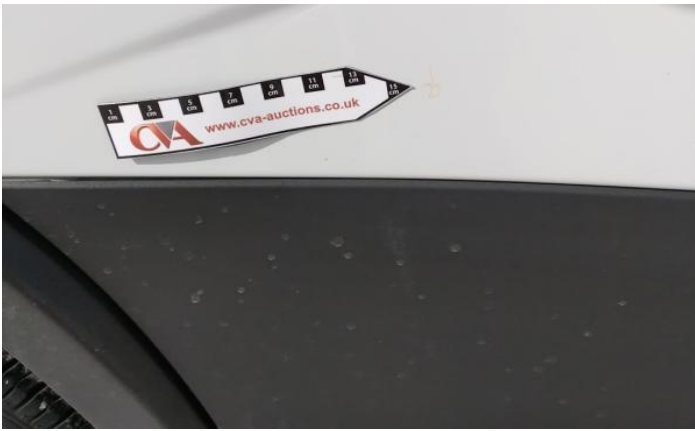
3: Bumper Front Scratched Over 100mm Thru Paint
