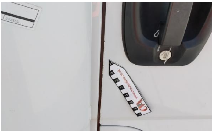
5: Door nsf Scratched Up To 25mm Thru Paint
