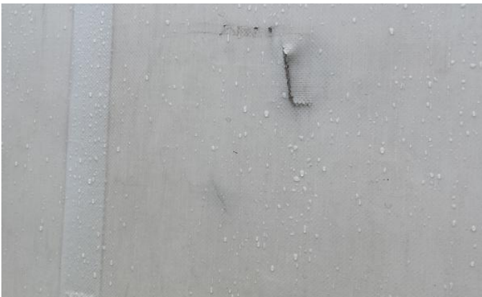
5: Wing osf Cracked Replace
