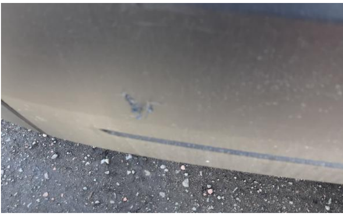
3: Door osf Dented With Paint Damage
