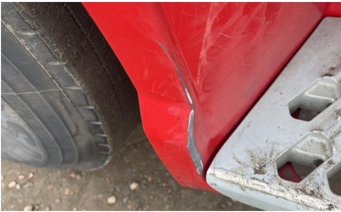
3: Wing osf Scratched Over 25mm Not Thru Paint
