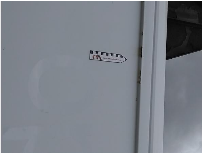
11: Qtr Panel osr Rusted Over 5mm
