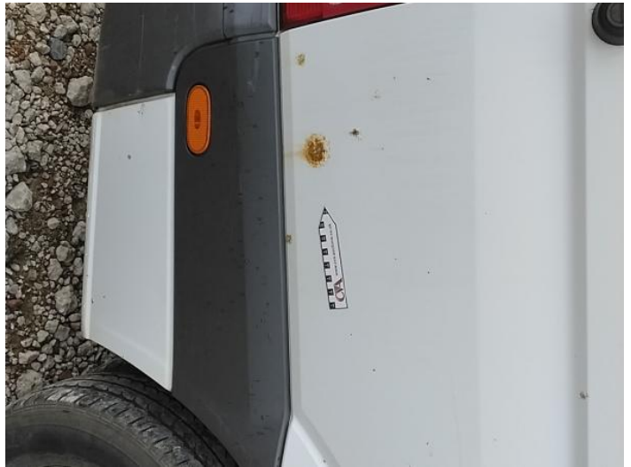
12: Qtr Panel osr Rusted Over 5mm
