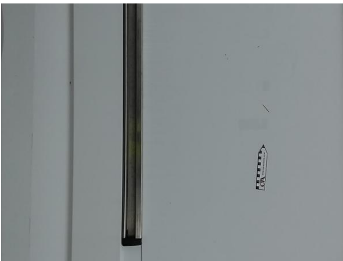
7: Qtr Panel nsr Rusted Over 5mm
