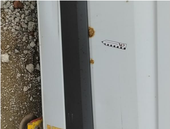
15: Qtr Panel osr Rusted Over 5mm
