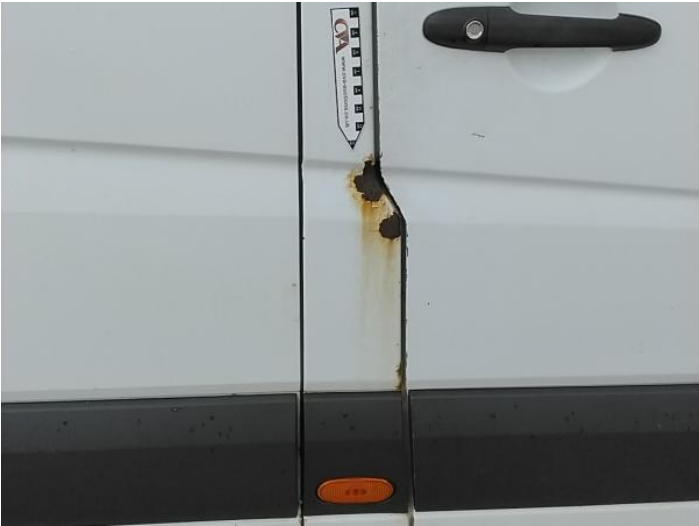
16: B Post os Rusted Over 5mm
