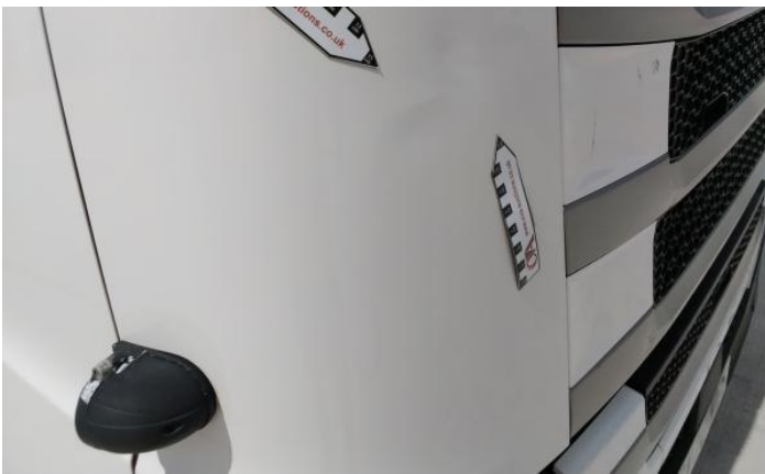
3: Bumper Front Dented Over 2 UpTo 10mm
