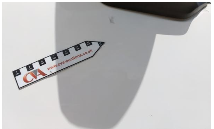
4: Bonnet Scratched Over 25mm Thru Paint
