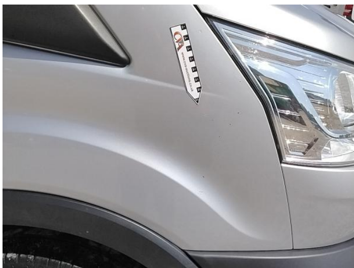
1: Wing osf Scratched Over 25mm Thru Paint
