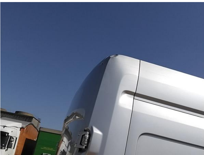
19: Qtr Panel osr Dented With Paint Damage
