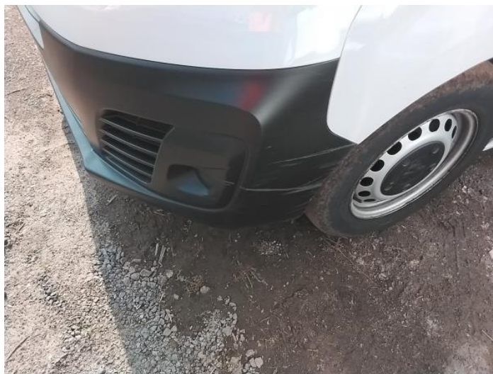
2: Bumper Front Scratched Over 100mm Thru Paint
