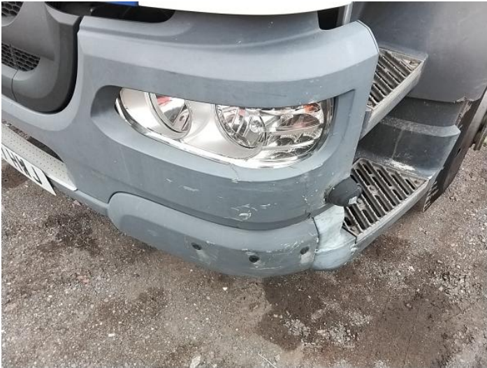
3: Panel Front Cracked Replace
