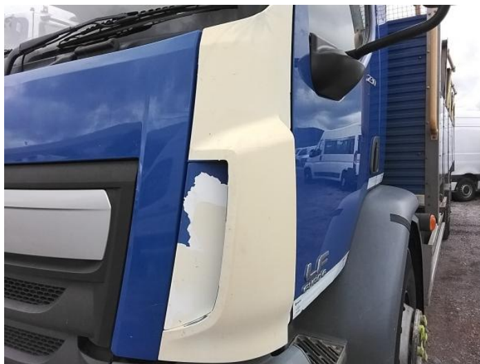
2: Panel Front Scratched Over 25mm Thru Paint
