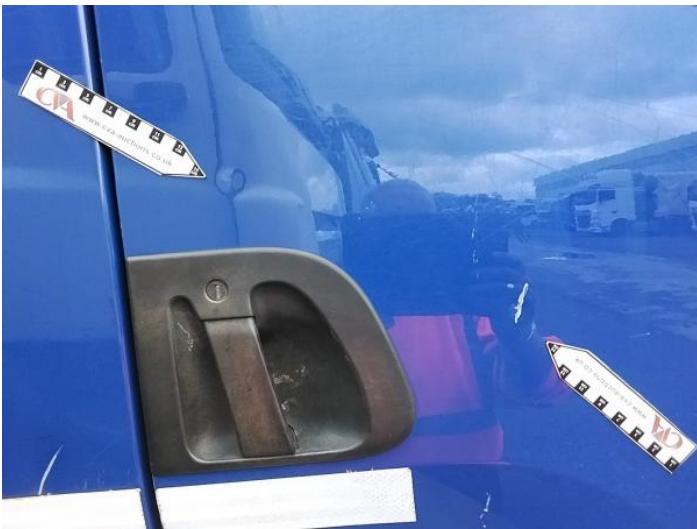
5: Door osf Dented With Paint Damage
