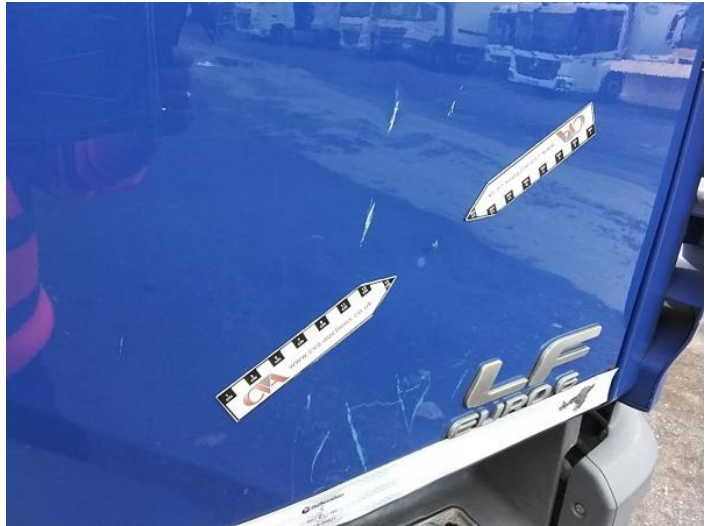
4: Door osf Dented With Paint Damage
