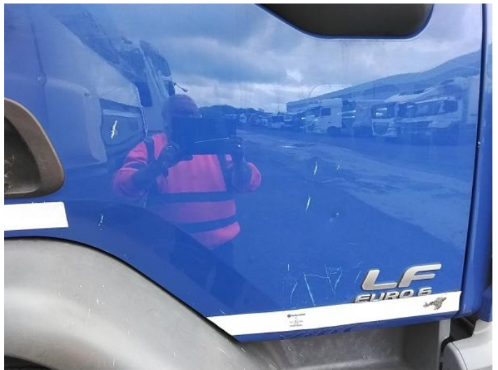
6: Door osf Scratched Over 25mm Thru Paint
