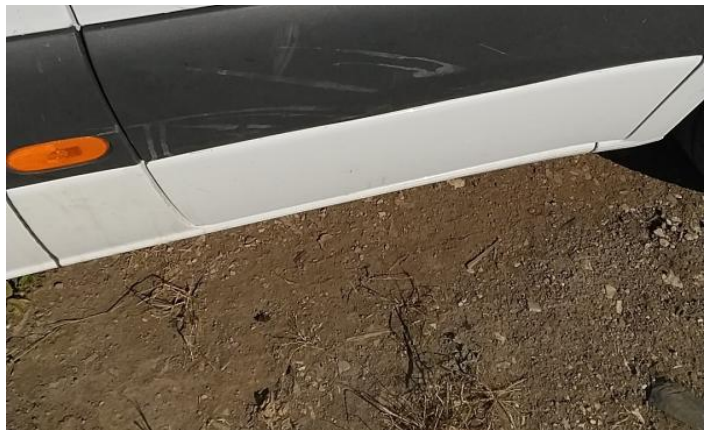
12: Qtr Panel osr Dented With Paint Damage
