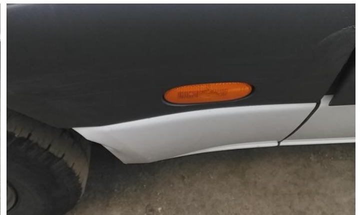
18: Qtr Panel osr Dented Over 30mm
