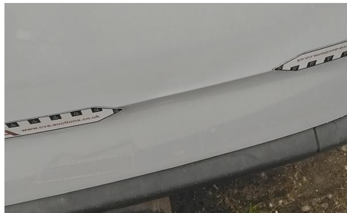
15: Door nsr Dented Over 30mm
