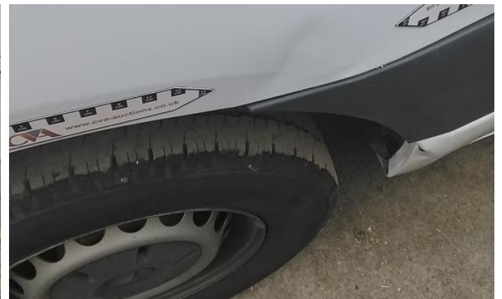
16: Door osr Dented With Paint Damage
