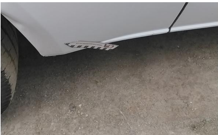
17: Door osr Dented Over 30mm
