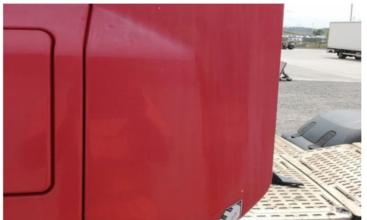
6: Door nsf Poor Previous Repair Poor Colour
