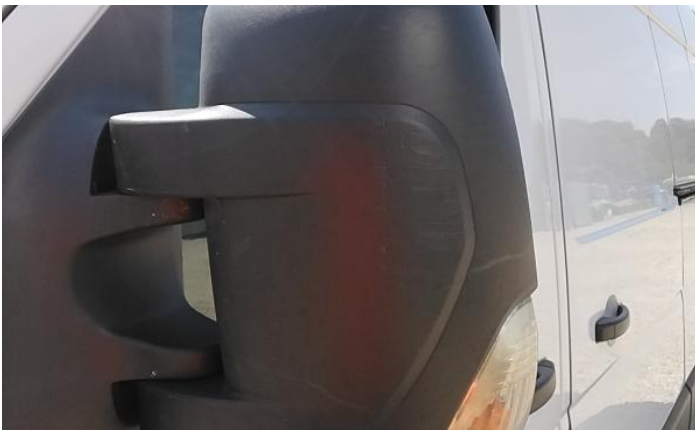
5: Bumper Front Moulding Scuffed (Unpainted) Over 100mm
