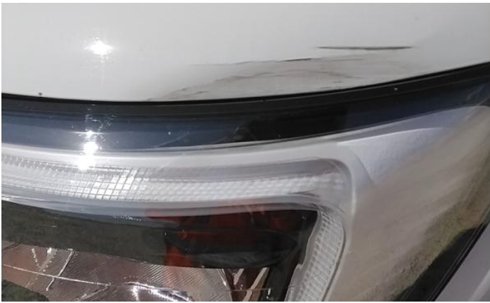
3: Bumper Front Moulding Scuffed (Unpainted) Over 100mm
