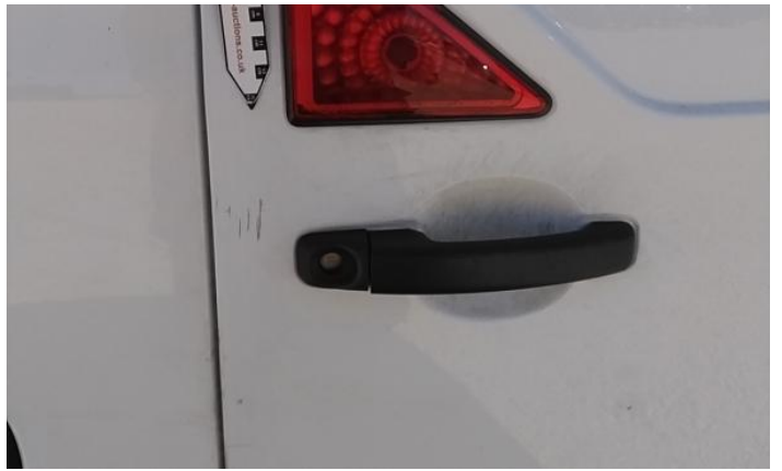
10: Door Moulding nsr Scuffed (Unpainted) Over 100mm
