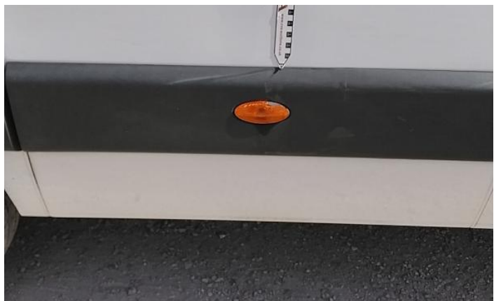
12: Door osr Scratched Over 25mm Thru Paint
