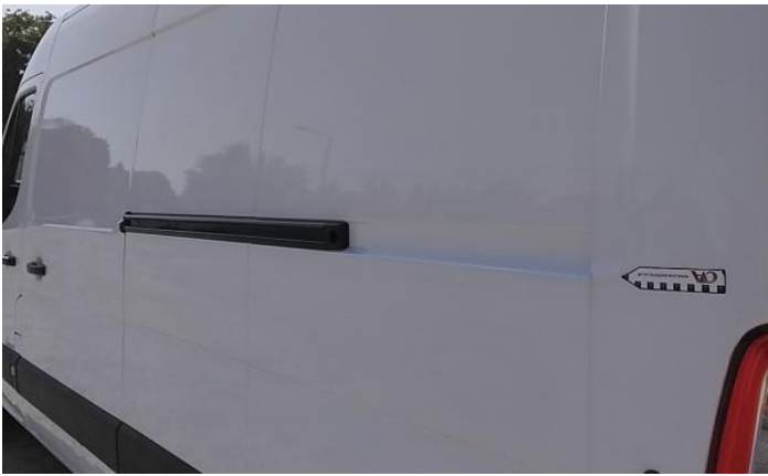
9: Door nsf Scratched Over 25mm Not Thru Paint
