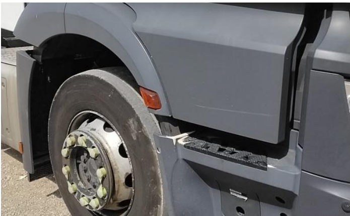
5: Wing Front Arch Extension ns Scuffed (Unpainted) Over 100mm
