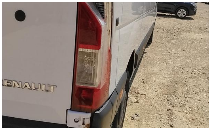
10: Door nsr Dented With Paint Damage
