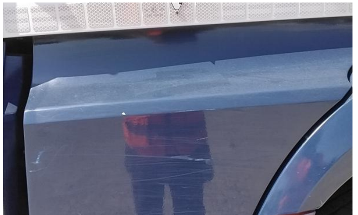
6: Wing nsf Scratched UpTo 25mm Thru Paint
