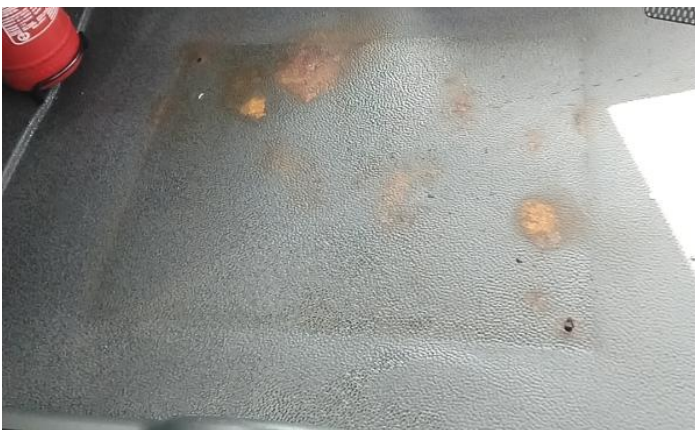
5: Wing osf Scratched Over 25mm Thru Paint
