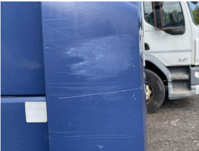
11: Wing osf Scratched Over 25mm Thru Paint
