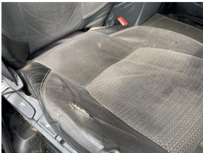
1: Seat Base Cover osf Torn Over 3mm
