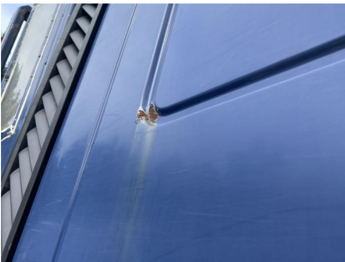
13: Qtr Panel osr Rusted Over 5mm
