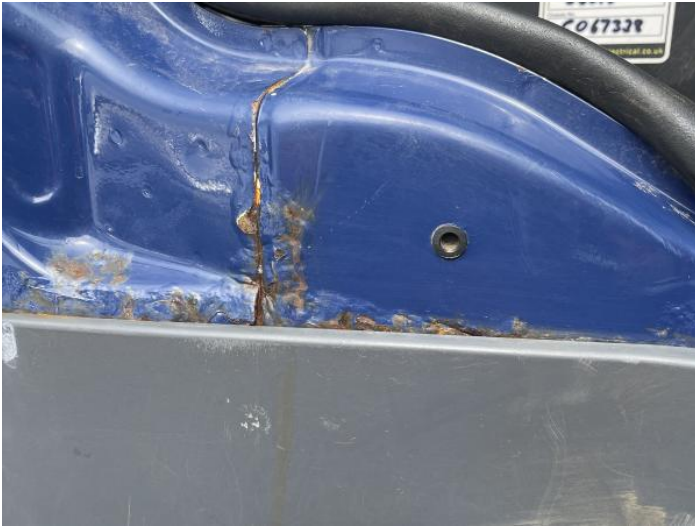
3: Sill os Rusted Over 5mm
