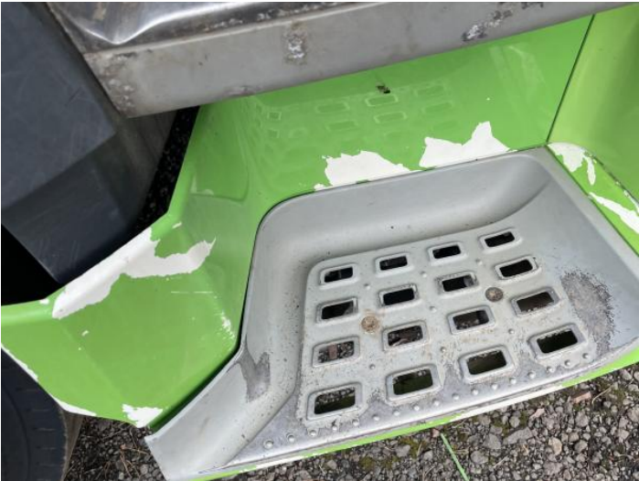
4: Door Moulding osf Scratched (Painted) Over 25mm Thru Paint
