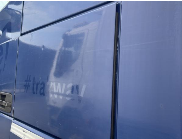
17: Qtr Panel nsr Dented Over 30mm
