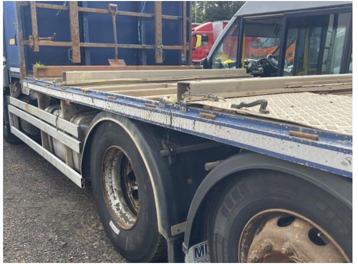
16: Qtr Panel nsr Rusted Over 5mm
