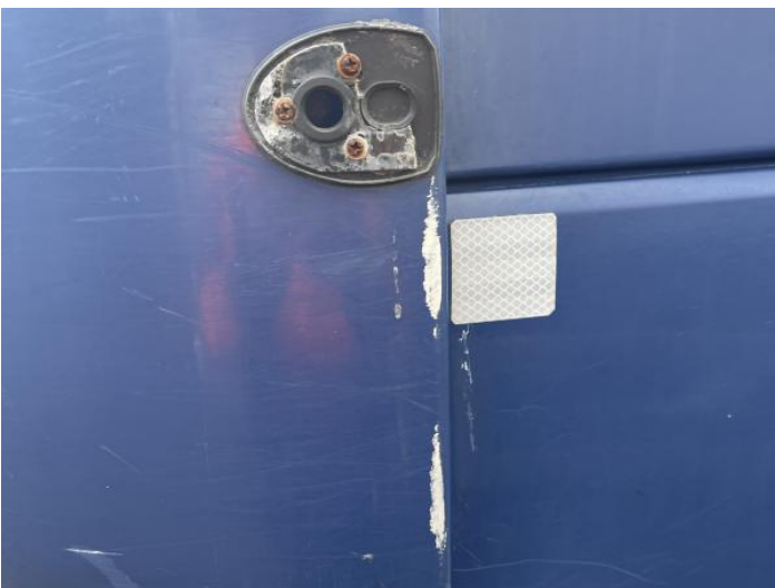
19: Wing nsf Scratched Over 25mm Thru Paint
