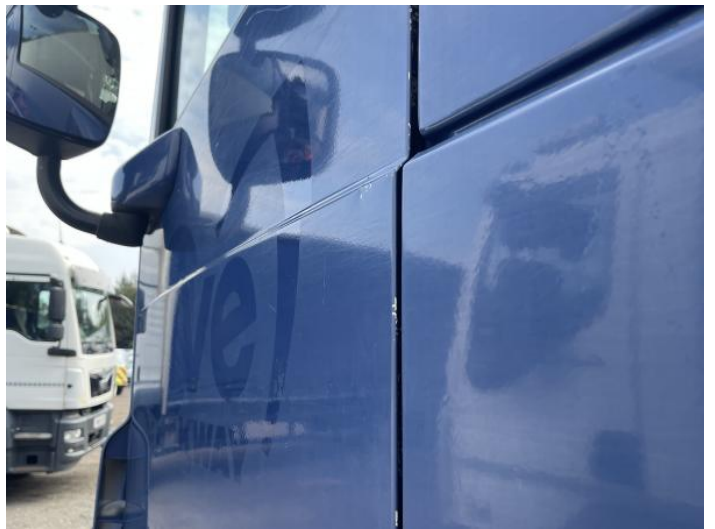
18: Door nsf Dented Over 2 UpTo 10mm
