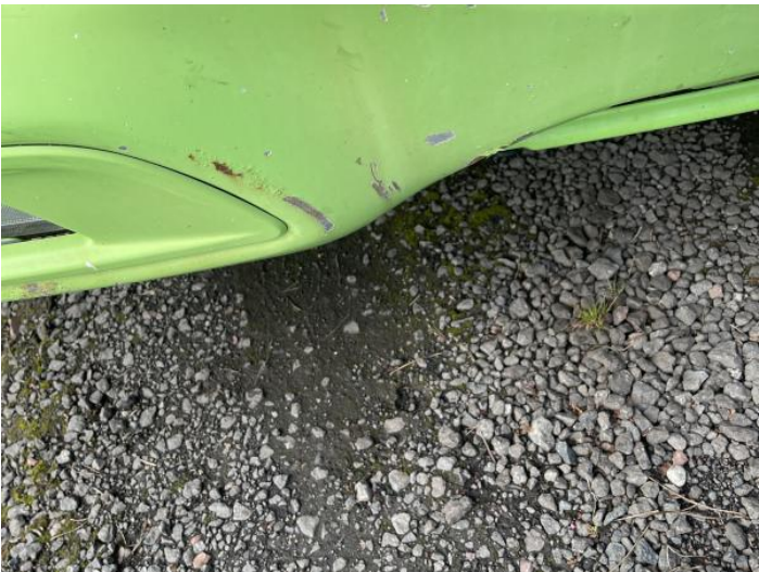
8: Bumper Front Scratched 25 to 100mm Thru Paint
