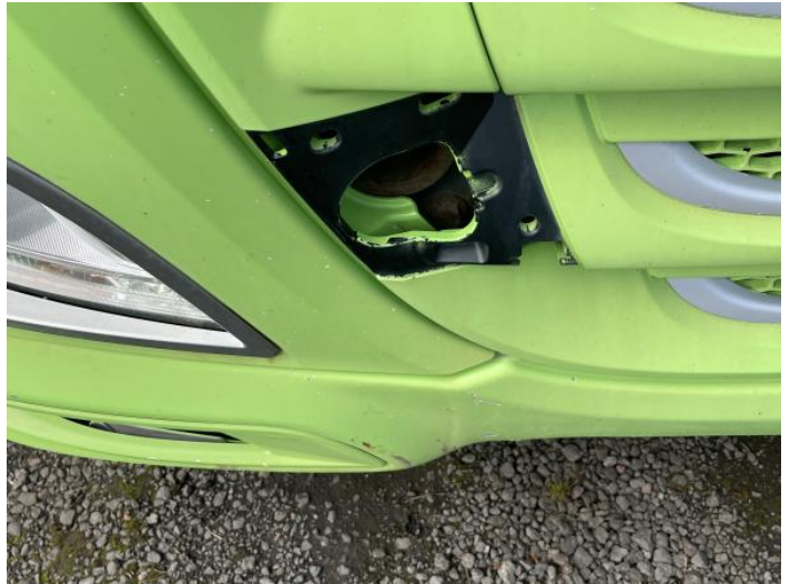
10: Front TowEye Cvr Missing Replace
