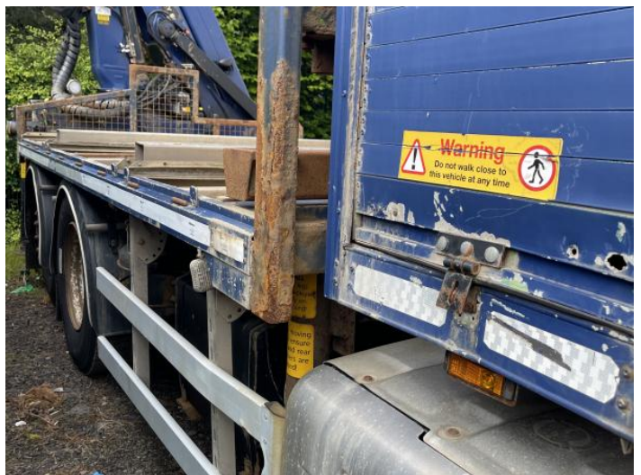
14: Qtr Panel osr Rusted Over 5mm
