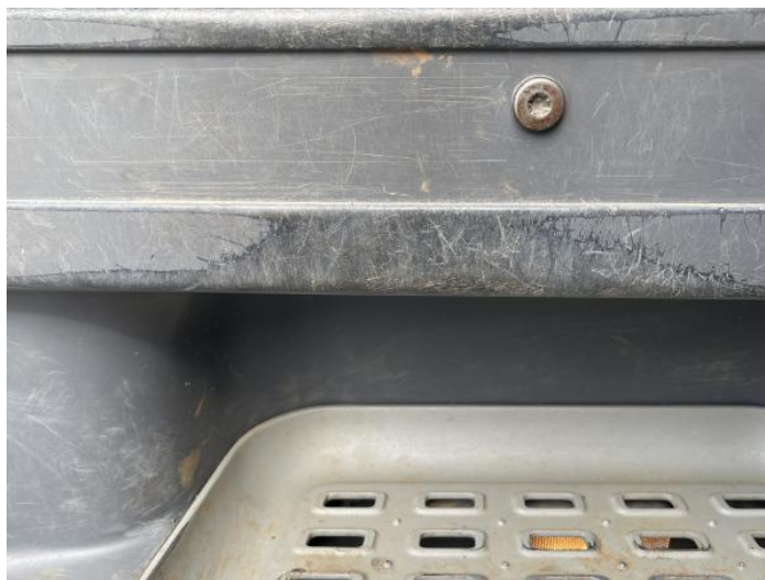
2: Door Moulding osf Scuffed (Unpainted) Over 100mm
