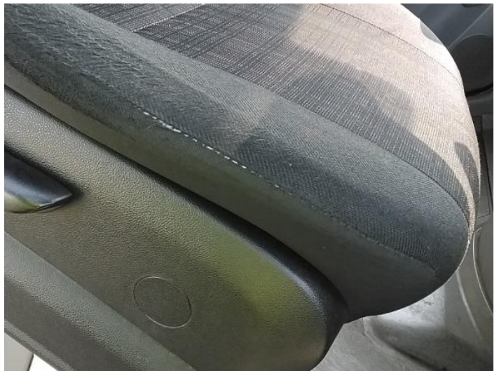
12: Seat Base Cover osf Torn Over 3mm
