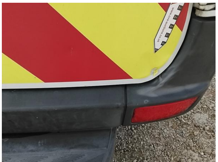
8: Door osr Dented With Paint Damage
