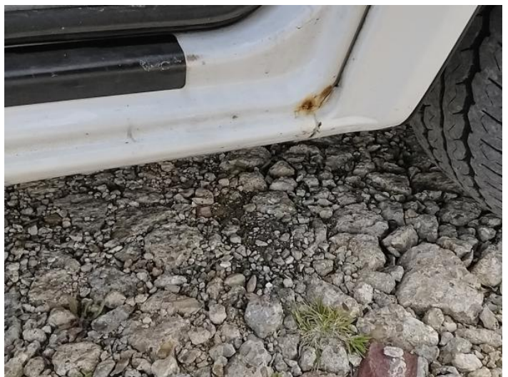
14: Sill os Rusted Over 5mm
