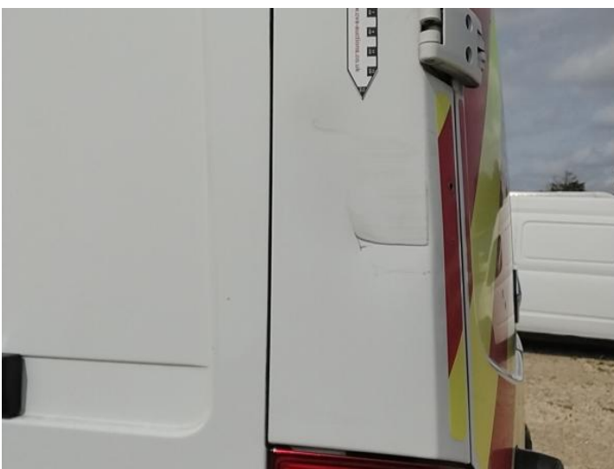
7: Qtr Panel nsr Dented With Paint Damage
